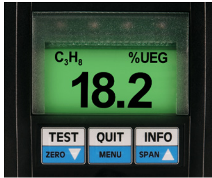
CC28 D with display and pushbutton interface
