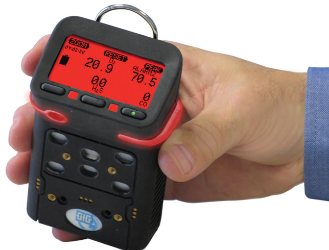
Figure 2: Hand-held multi-sensor instruments are compact, easy-to-use and capable of being equipped with an increasing number of substance-specific as well as broadly responding sensors.
