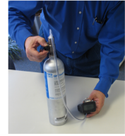
Figure 1: Performing a functional “bump test” by exposing the instrument to test gas takes only a few seconds to perform.
