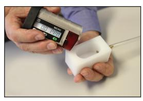
After inserting the instrument into the calibration adapter, open the regulator valve to begin flowing HCl gas to the instrument. When the reading reaches 5.0 ppm, or has run for two minutes, THEN initiate the AutoCal "Gas" calibration step. Newer sensors respond more quickly than older and may reach 5.0 ppm, or more, within one minute.
