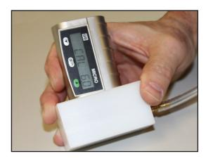
The instrument will wait for the sensor to reach its final stable reading, then adjust the reading to match the concentration of the calibration gas.
